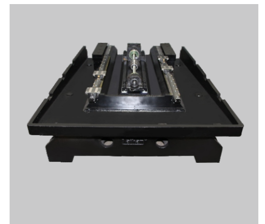
Best slanting angle base and special designed chip deflector system, avoid the chip pile up, good for the cutting fluid counter flow smoothly.
