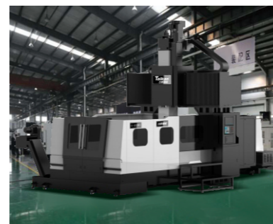
The production workshop of gantry machining center
