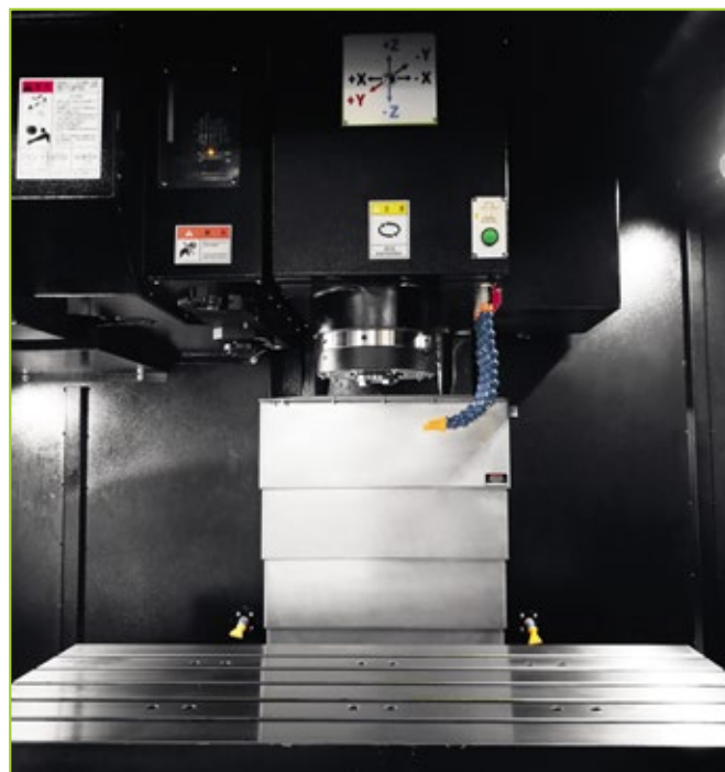
Keyarrow telescopic covers in all axes
