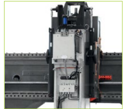
Hydraulic balancing system in Z axis
