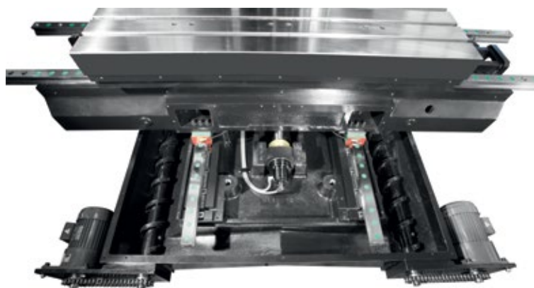
Two screw type chip conveyors in Y-axis (VF1100 & VF1300 & VF1500)
