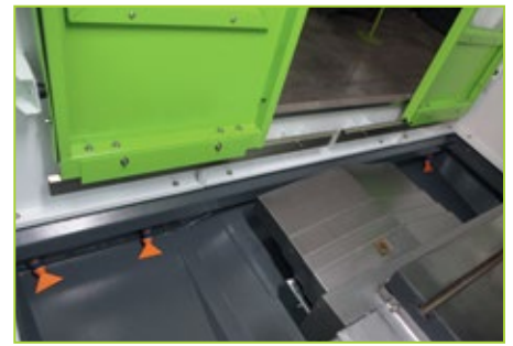
Chip flushing system
